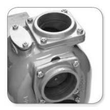
Standard inlet and outlet ports are BSP (GAS) threaded (up to 4"), on request also NPT; the ports are screwed on the casing to easily disconnect the pipes.
