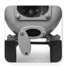
Clean out cover it is used to empty the casing, especially in the colder months, to prevent the water from freezing inside.
