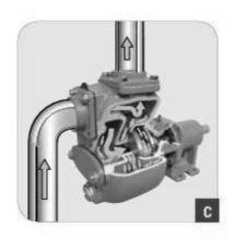
The S series pumps are centrifugal and self-priming. The impeller with open blades allows a wide passage of solids. With this kind of pump you can handle wastewater also with corrosive and viscous liquids containing solids in suspension, abrasive powders, even if there are air bubbles.
