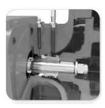
**External flushing seal**
