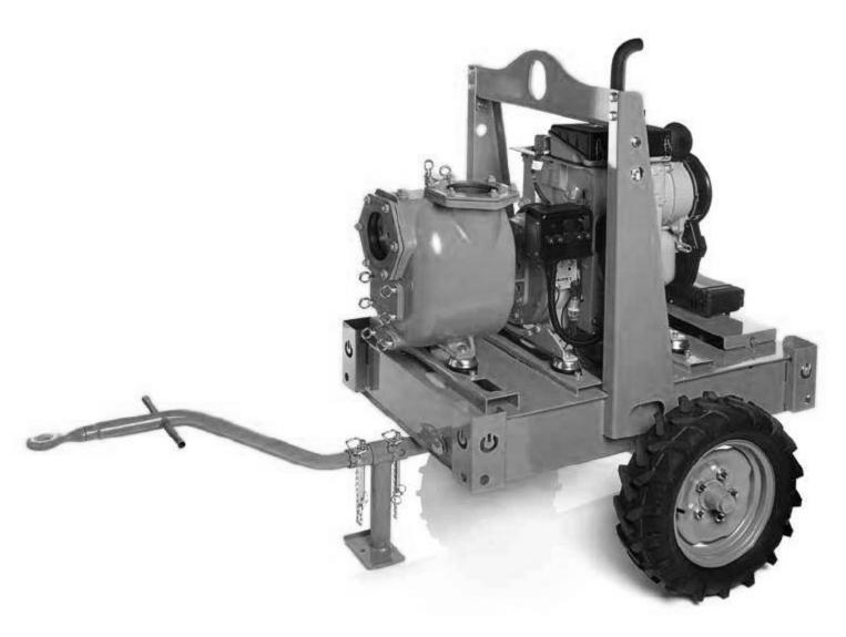
6" cast iron pump, close coupled to diesel engine, on trailer with tractor profile wheels, large capacity tank for heavy and continuous use. The lifting and towing hooks allow various types of handling.
