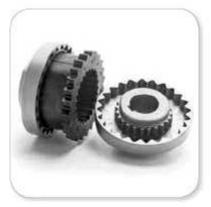
SX coupling elastic coupling to dampen noises caused by the engine and by the irregular flow. The central elastic element breaks in the event of a blockage of the pump, protecting the motor and the gear box.
