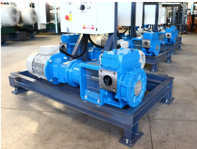
Pump skid with control panel
